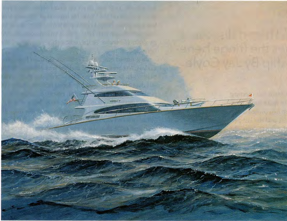
STABLE PLATFORM: The Quantum units on Mary P will fold flush into hull recesses when necessary; at that point, a computer-controlled system will activate the trim tabs for high-speed roll stabilization.
