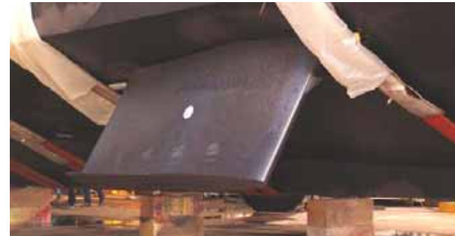
Above & Left: The Trinity yacht 'Fox Harb' y Too' launches with her Quantum Zero Speed™ Stabilisers clearly visible.
